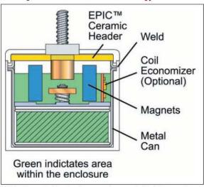
making an exact-shaped chamber to manage the arc can be tricky. The coil economizer is within the sealed enclosure.
