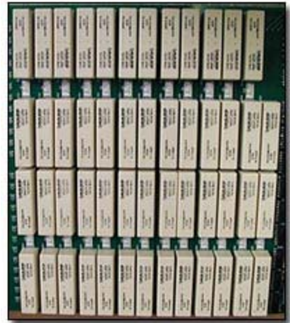
This is the wrong way to do it! Relays are too close and not alternated end-to-end
